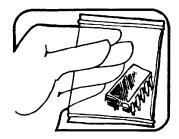
Use anti-static containers for handling and transport.
